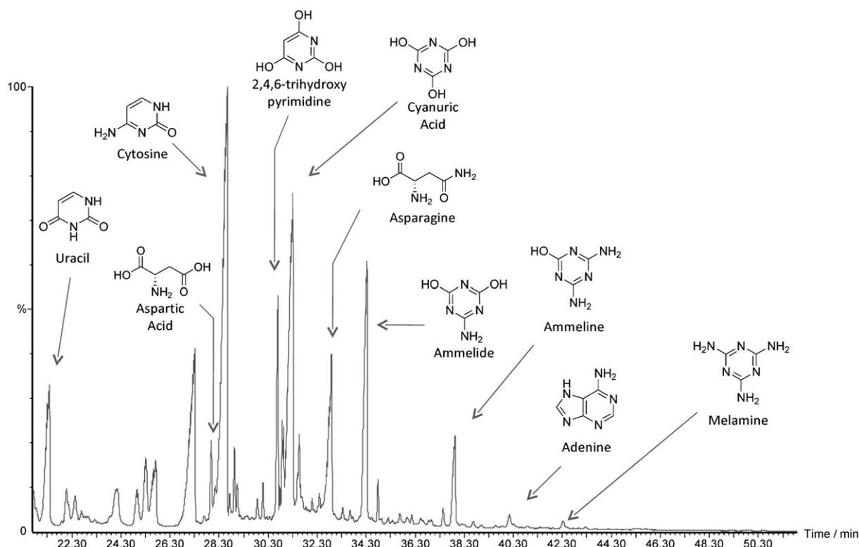
Figure 2. Gas chromatogram showing the trimethylsilyl derivatives of pyrimidines and triazines obtained from spark discharges between a  $\text{CH}_4/\text{N}_2/\text{H}_2$  atmosphere and a 0.1 M urea solution subjected to freeze–thaw cycles. Residual urea (not shown) appears as a strong peak (urea–TMS derivative;  $m/z$  204, 189, 147, and 73) at a retention time of 19 min.
