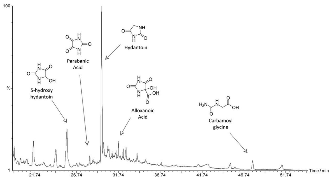
Figure 3. Gas chromatogram showing the trimethylsilyl derivatives of hydantoin derivatives obtained from spark discharges between a  $\text{CH}_4/\text{N}_2/\text{H}_2$  atmosphere and a 0.1 M urea solution at room temperature. Residual urea (not shown) appears as a strong peak at a retention time of 19 min.
