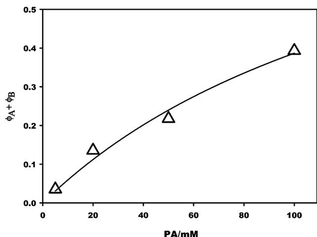
**Figure 8.** Sum of the apparent quantum yields of formation of **A** and **B**,  $\phi_A + \phi_B$ , vs  $[\text{PA}]$  in the photolysis of deaerated aqueous PA solutions at 293 K. Quantum yields normalized to the condition  $(\phi_A + \phi_B) \rightarrow 1$  as  $[\text{PA}] \rightarrow \infty$ .
