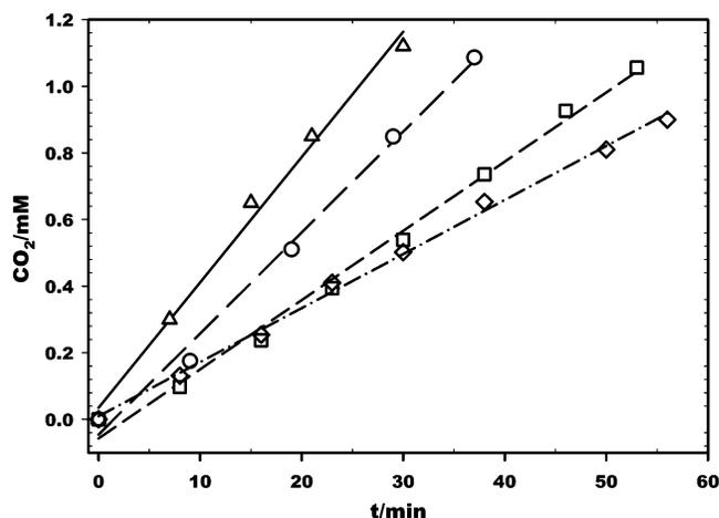
**Figure 1.** CO<sub>2</sub>(g) evolution during the 313 nm photolysis of deaerated aqueous 0.1 M PA solutions at 293 K in the presence of various TEMPO initial concentrations: 0 (Δ), 0.50 (○), 1.36 (□), 1.71 mM (◇).
