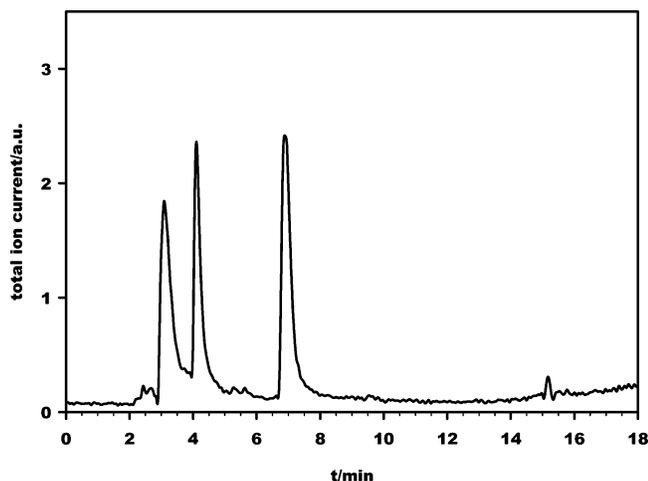
**Figure 4.** Liquid chromatogram of deaerated 0.1 M PA solutions after photolysis for 1 h. The species eluting at 3.1, 4.1, and 6.9 min are detected as 87, 177, and 175 Da anions, respectively, via negative ion ESI-MS.
